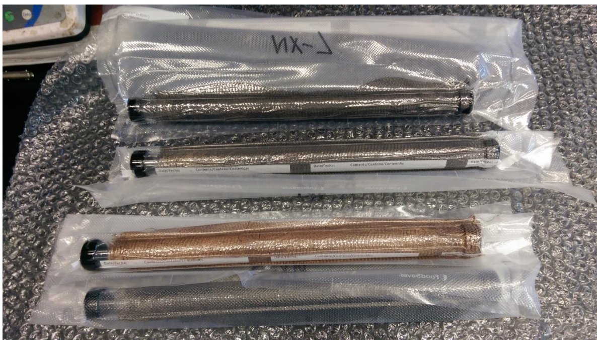
Figure 15. Vacuum Sealed Scrim Blanket Samples
