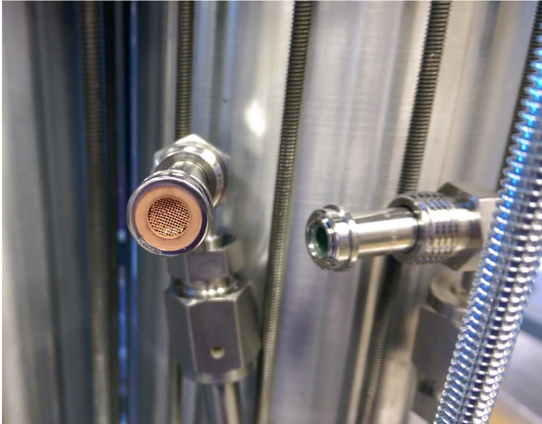
Figure 17. Copper Mesh to Protect the Hotwire
