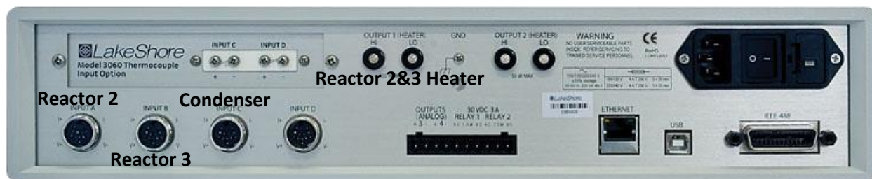
Figure 20. Lakeshore 336 Temperature Controller #2 Wiring Diagram
