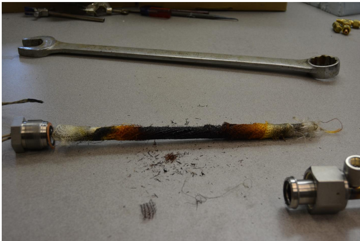
Figure 24. Control Scrim Blanket destroyed by pyrolysis.
