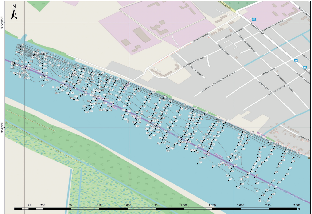
⤴ Image 19. The results of measuring the depth and bathymetry of the bottom at the Kiliya branch, 20-18 km in June 2019.
