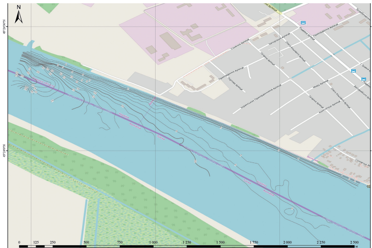
⤴ Image 19. The results of measuring the depth and bathymetry of the bottom at the Kiliya branch, 20-18 km in June 2019.
