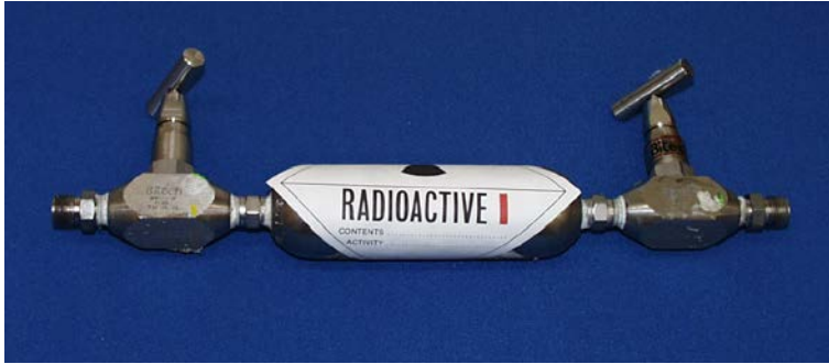
FIG. 5. Container for transportation and flow through injection of beta emitting tracers.
