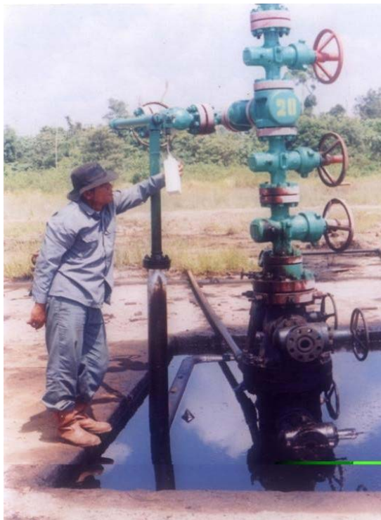
FIG. 18. Manual sampling at the well head of an oil well.
