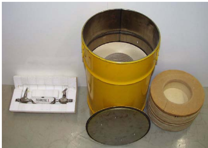
FIG. 6. Drum lined with shock absorbant material for transportation of the container.
