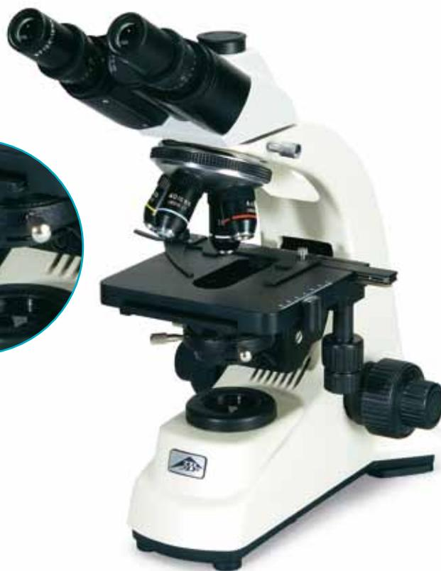
Microscopes U30712 and U30713 provide for binocular or monocular viewing as well as allowing simultaneous fitting of a camera for photographic or video recording of the image.
