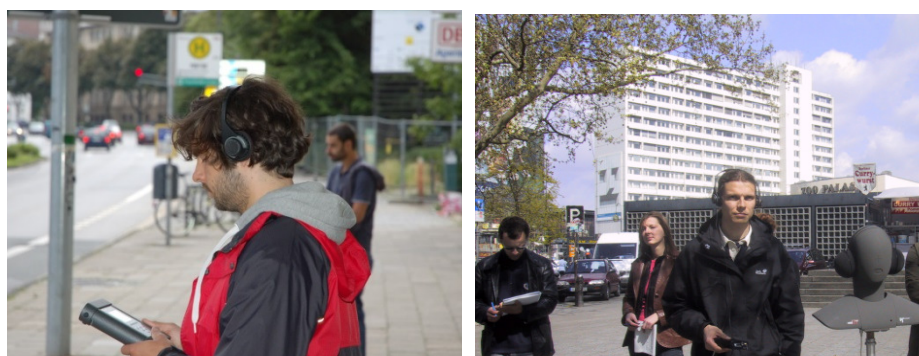
Figure 3 – Binaural measurement during soundwalk. Left: Binaural recording via binaural headset; right: Binaural recording via artificial head measurement system and binaural headset
