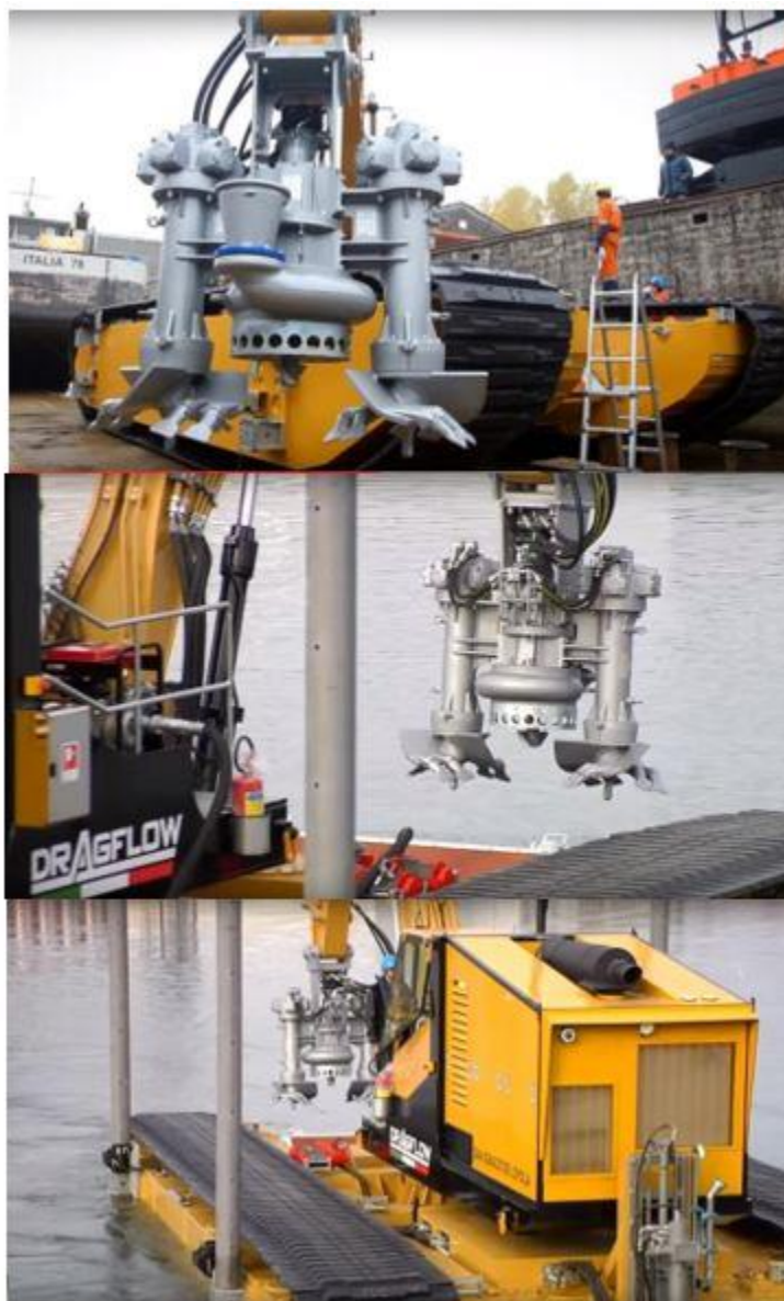
Figura 6 Hydraulic pump HY85/160HC
