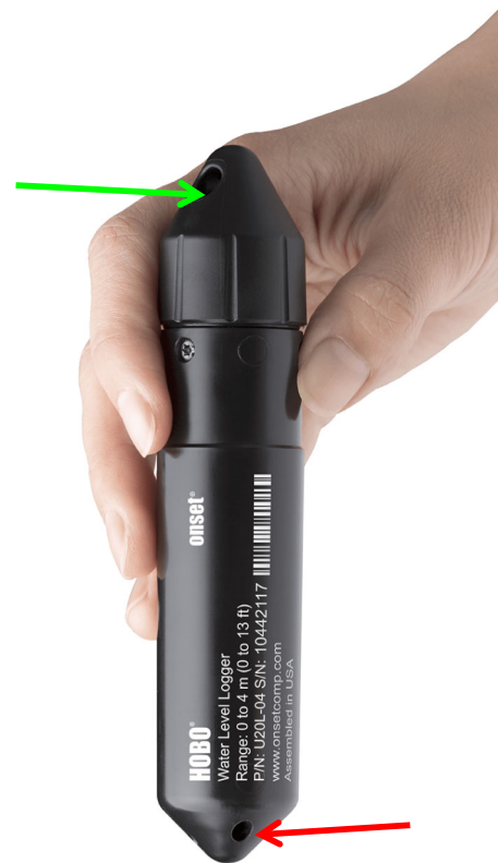
Fig. 6 Pressure transducer, which measures the height of the water column above the pressure sensor, shown by the red arrow on the left side of the figure above. This field instrument is also equipped with a temperature thermistor, which measures the temperature of the groundwater. Under most conditions, the transducer is hung vertically in the well by a cable through the cap, identified by the green arrow . Water level and temperature data are stored internally in the instrument at a predetermined time interval, typically every 5 min. Data are downloaded periodically by removing the instrument from the well, unscrewing the water-tight cap and connecting it to an optical reader interface attached to a field laptop. Once downloading is complete, the instrument is reset, reinstalled in the well, and the water level is measured with an electric tape to verify the exact water level. The entire process is documented in a field notebook to facilitate data interpretation
