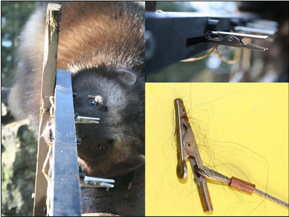
Figure 6. Device for snagging wolverine hair using alligator clips.
