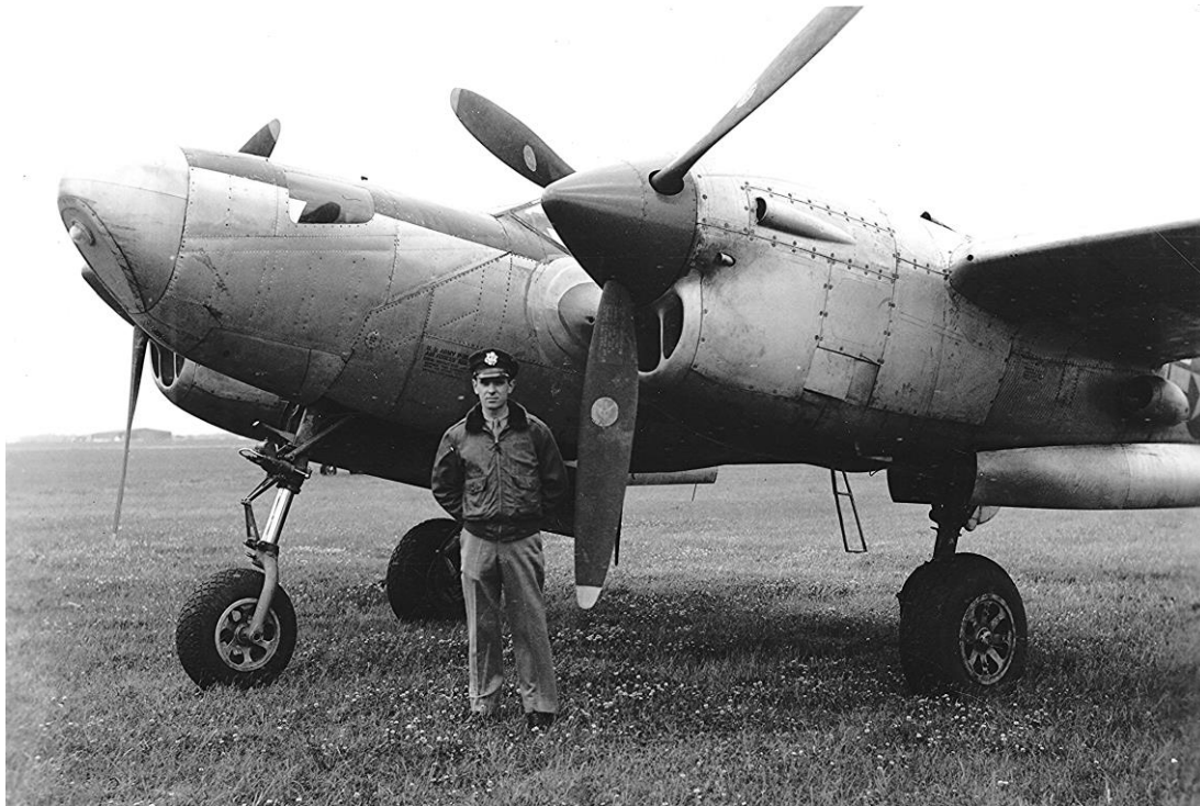
Figure 18. Lt Holt, one of the radar observers assigned to the three P-38Js operated by the 36th BS, is seen posing next to one of his mounts. The P-38J “Droop Snoot” modification was used for formation bombing by other fighter aircraft; the electronic modification used by 100 Group and later the 36th BS removed the Norden bombsight and added a receiver, whose antenna is seen here mounted on the flat bomb aiming panel. (Air Force Historical Research Agency)
