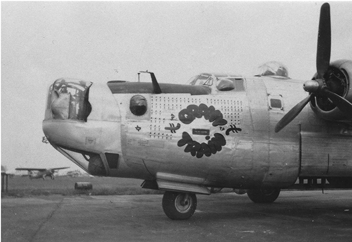
Figure 10. 36 th BS B-24J-5-FO Liberator #42-51546 R4-L Gravy Train with a healthy mission log painted on her nose waits in the English gloom between sorties. What appears to be a Carpet antenna is just aft of the nose wheel. (Stephen Hutton)
