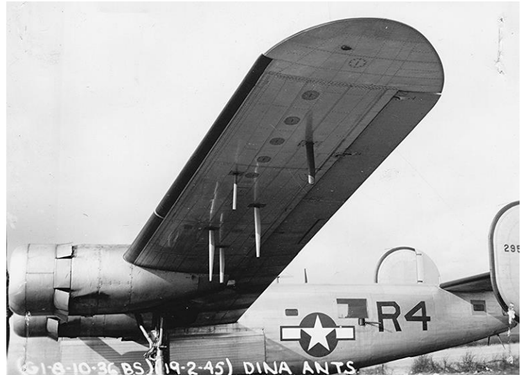
Figure 5. Most of the jamming antennas were fitted to the underside of the wings of 36 th BS aircraft, though Jackal antennas were carried under the fuselage just forward of the tail turret and Carpet antennas under the fuselage aft of the nose wheel. This photo depicts the Dina antennas under the outer wing. (Air Force Historical Research Agency)
