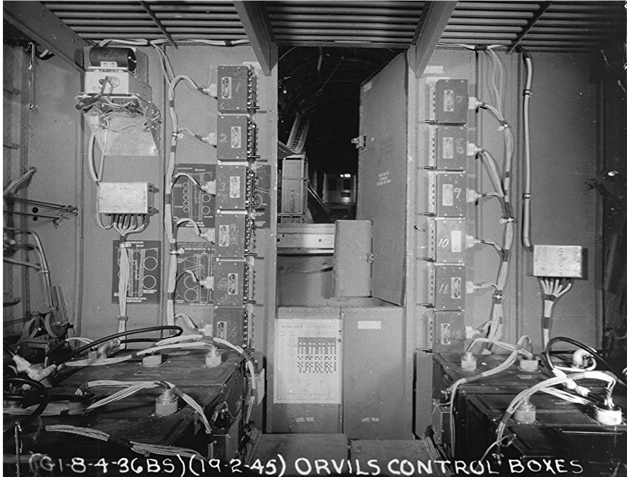
Figure 19. The Orvils started to replace the Dina as the primary VHF jammer with the 36 th BS in February 1945. Orvils control boxes were mounted on either side of the bomb-bay door of squadron aircraft with transmitters on a wooden floor as depicted in the foreground. The modified VHF SCR-522 radios used a Gaston gas tube, seen at the upper left-hand corner of the picture, as a noise source with a stage of amplification to modulate all twelve transmitters. (Air Force Historical Research Agency)
