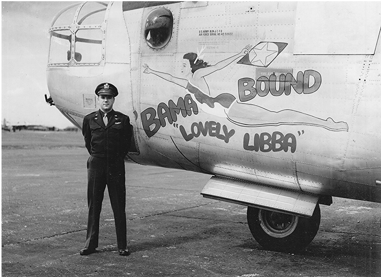
Figure 20. Lt. Col. Robert F. Hambaugh, 36 th BS commander and a native of Birmingham, Alabama, poses in front of B-24J-2-FO s/n 42-50622, BAMA BOUND /' LOVELY LIBBA '. This Liberator has had its nose turret replaced by glazing reminiscent of modifications seen on 801 st BG (P) Carpetbagger B-24s and apparently was the only aircraft in the squadron so modified. In December 1944 this aircraft was modified into one of the squadron 'ferret' search aircraft, though around the time this photo was taken in April 1945 the search equipment had been removed. (Air Force Historical Research Agency)
