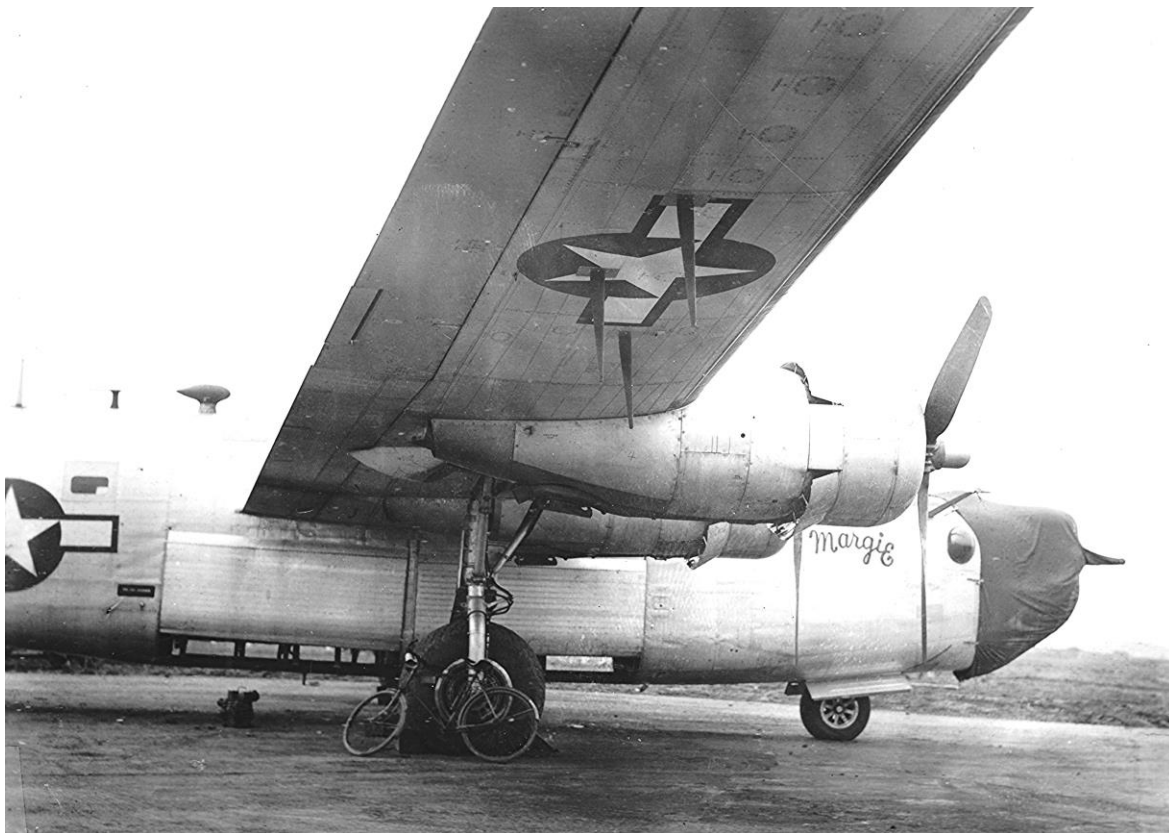
Figure 17. Close up of the Orvils VHF jamming antennas fitted to the starboard wing of 36 th BS B-24H-25-FO Liberator #42-95221 nicknamed Margie (originally READY N' ABLE ). Orvils was a VHF screening jammer that used an SCR-522 radio modified to produce modulated noise; in February “Margie” was fitted with six of these jammers. (Stephen Hutton)
