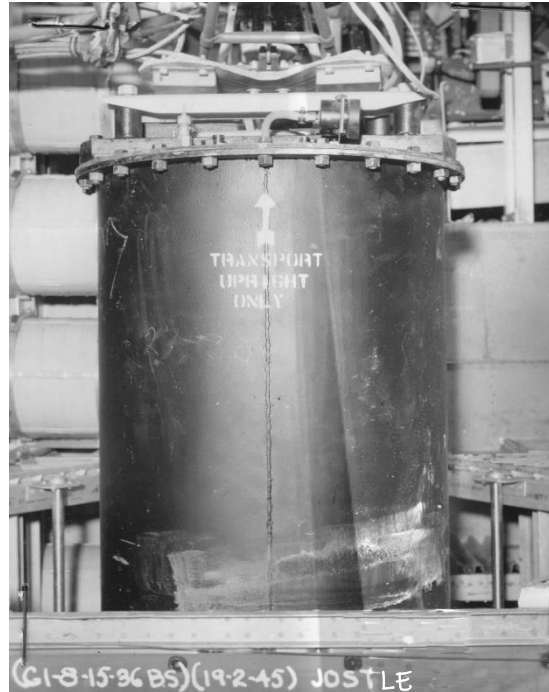
Figure 13. The British Jostle jammer was experimented with on two aircraft and found superior to the Jackal and plans were ready to procure more if the need arose. The 600 pound Jostle transmitter is shown mounted in the ball turret position of a squadron B-24 aircraft. To remove the transmitter, the B-24 had to be positioned over a pit dug on the edge of the hard-stand which the Jostle could be lowered into. (Air Force Historical Research Agency)
