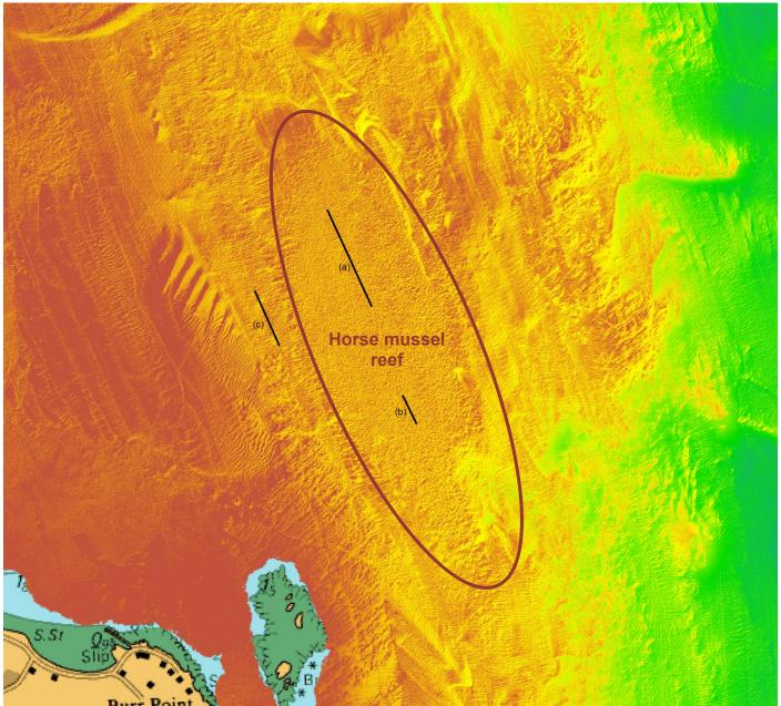
Figure 3.20. Distinctive "rippled" bathymetric signature from 2m horizontal resolution multibeam off Burial Island. Bathymetric profile positions indicated by black lines.
