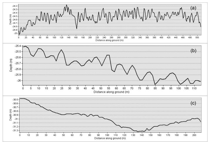
Figure 3.19. (a) and (b): Bathymetric profiles across known *Modiolus* reef area at Craigbrain, showing rippled structure, and (c) Bathymetric profile in area adjacent to *Modiolus* reef (all profiles in NNW to SSE orientation, with profiles marked on Figure 3.18 above).
