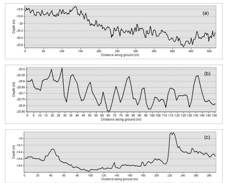
Figure 3.21. (a) and (b): Bathymetric profiles across known *Modiolus* reef area at Burial Island, showing rippled structure, and (c) Bathymetric profile in area adjacent to *Modiolus* reef (all profiles in NNW to SSE orientation, with profiles marked on Figure 3.20 above).
