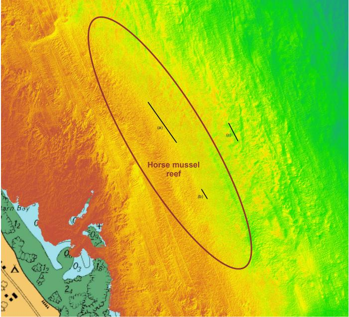
Figure 3.18. Distinctive "rippled" bathymetric signature from 2m horizontal resolution multibeam off Craigbrain. Bathymetric profile positions indicated by black lines.
