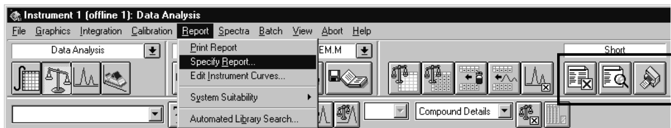
Figure 6 Report menu and smart icons (far right) in ChemStation Data Analysis view
