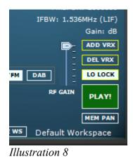
3. Hit the **Play** (Fig.8) button on the SDRuno Main panel and **Start** on the TCP Server Plugin window (Fig 8). Adjust the slider to broadcast every X milliseconds. I ran it at 100 ms.
