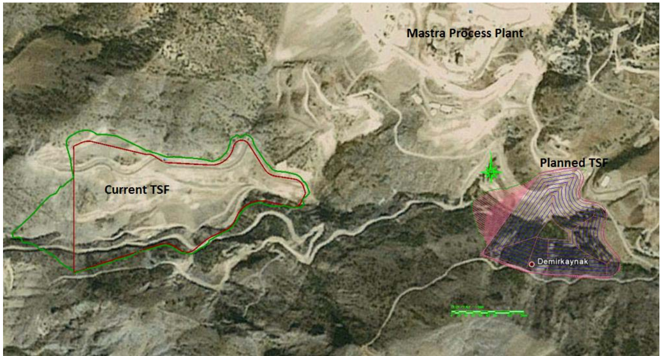
Figure 2.8.1: Mastra Tailings Storage Facility Plan
