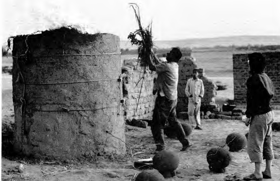
Figure 8.17. Throwing clean fuel onto the kiln top in order to decarbonise it. This marks the final stage in the firing of the kiln.
