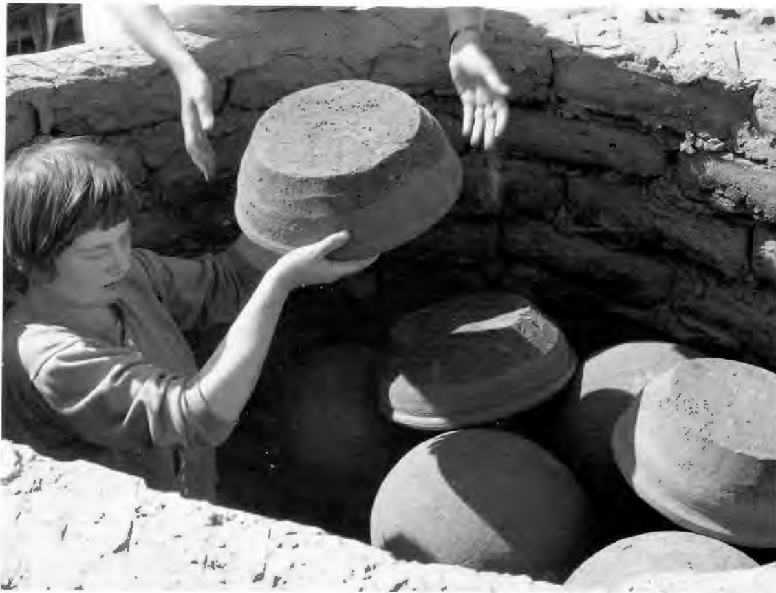
Figure 8.4. Catherine Powell loading the 1989 kiln for firing 1. Bowls are being placed in an inverted position over the inverted gidr below.
