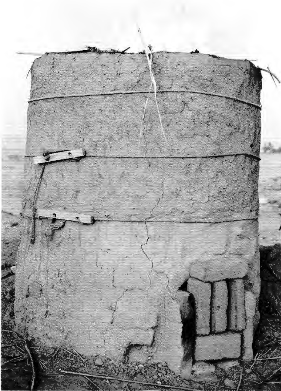
Figure 8.16. The kiln stoke hole is blocked during decarbonisation of the kiln top.
