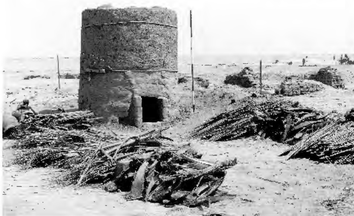
Figure 8.14. The 1992 kiln just before firing. The fuel can be seen in the foreground, divided into weighed piles according to which part of the branch it came from.
