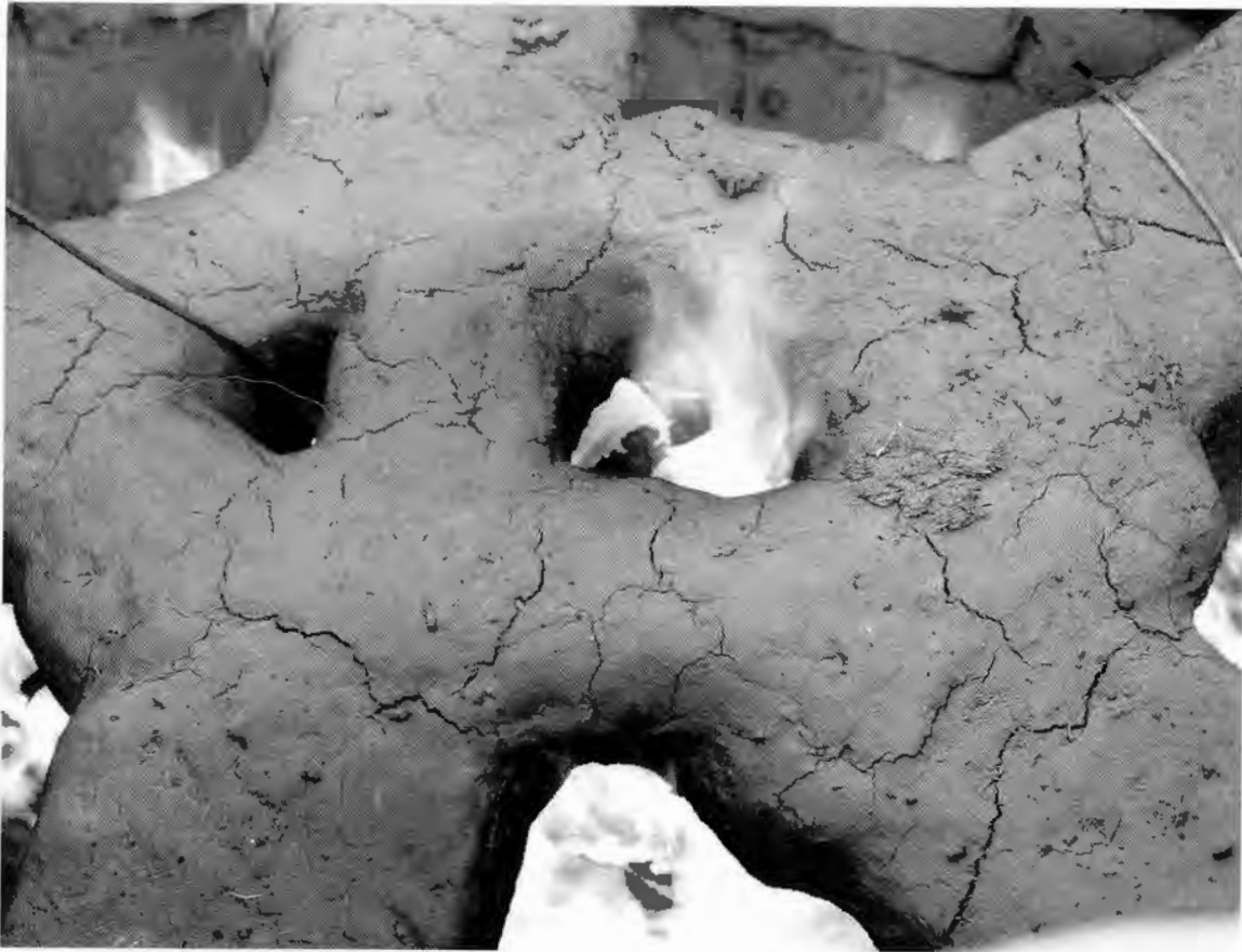
Figure 8.10. Burning out the former from the new fenestrated floor.
