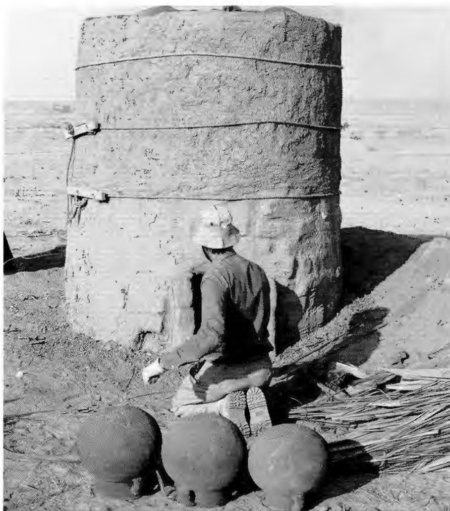
Figure 8.15. Firing the 1992 reconstruction. Note that for this firing three rope bands were used to help cope with the expansion of the kiln.
