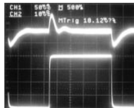
Figure 2. Step response of LT1158-based terminator
