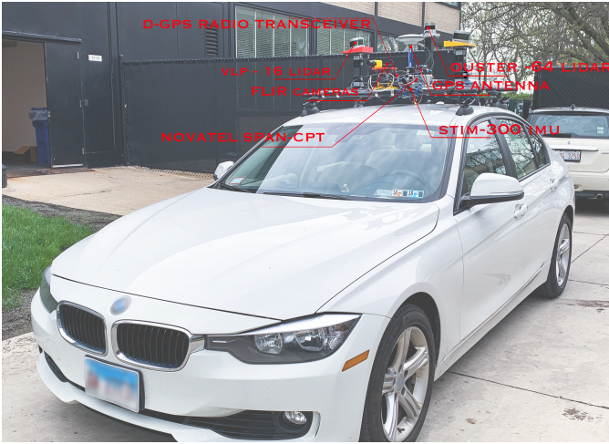
Fig. 5. The test setup used for the experiment. The sensor suite consists of STIM-300 tactical-grade IMU, two Velodyne VLP-16 lidars, one Ouster-64 lidar and Novatel SPAN-CPT DGPS attached to a roof-rack of a vehicle. For this experiment only the STIM-300 and Ouster lidar were used. Columns, tree trunks, and lamp posts are used as landmarks for localization.
