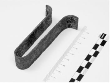
Figure 8: Stirrup for ceiling reinforcement found at the malting factory. Photo: Buchenau 2020.
