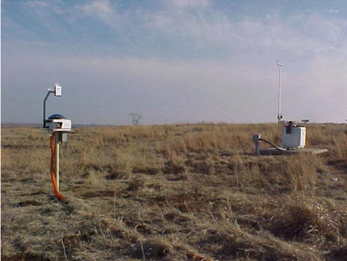
Figure 6. Picture Showing the Relative Closeness of the TSI (left) and WSI (right) at the SGP.
