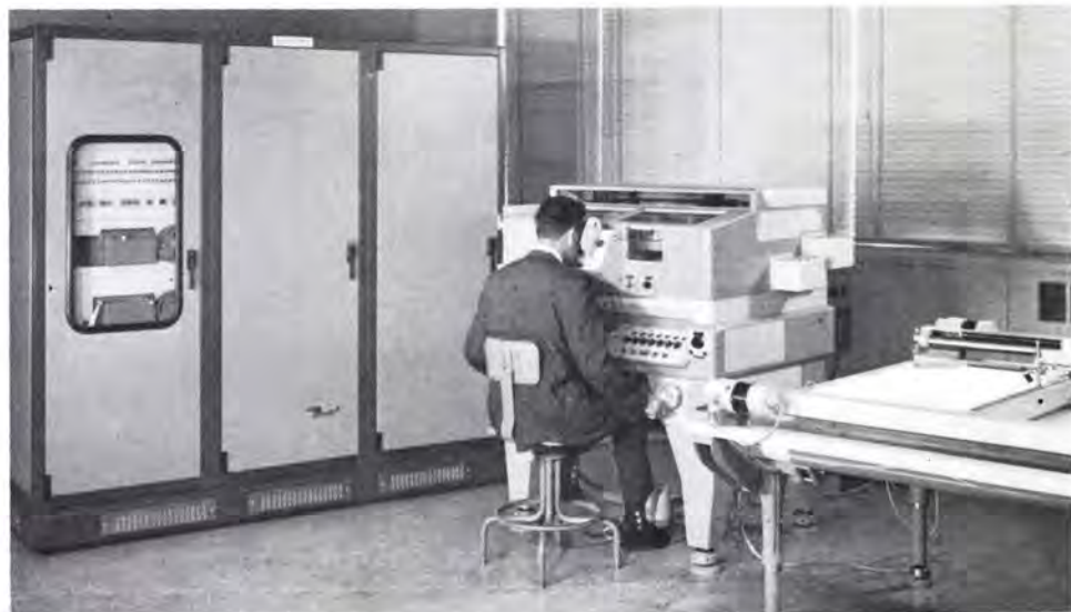
Fig. 3. The production model of the Analytical Stereoplotter AS-11A.
