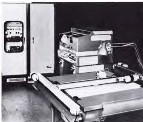
FIG. 2. The first Analytical Stereoplotter AP-1.
