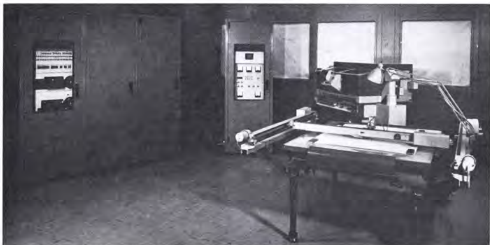
FIG. 5. The first Automated Analytical Stereoplotter AS-11B.
