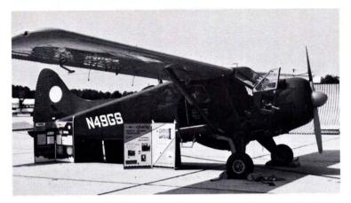
$F_{IG.}$  4. U.S. Geological Survey De Havilland Beaver with the AN/AAS 24 Thermal Infrared Imager.
