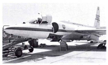
FIG.2. NASA Lockheed U-2 showing VINTEN RC-10 camera package for multispectral use.
