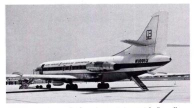
FIG. 5. Aero Service Goodyear Aerospace Aerospatiale Caravelle with pod containing Side-Looking Radar antenna under the aircraft.
