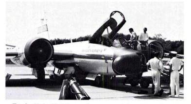
FIG. 3. NASA-RB-57E aircraft sensors include metric and multiband cameras, and the infrared system shown consisting of a scanner and a spectrometer/radiometer.
