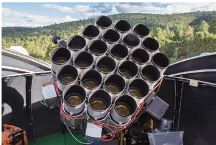
The 24-lens iteration of the Dragonfly Array. Image by Pieter van Dokkum, Yale University; website at www.dragonflytelescope.org .
