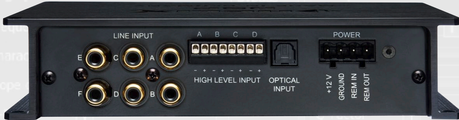
The HELIX DSP provides three sets of stereo preamplifier inputs (RCA/Cinch; A-F) and an optical stereo digital input. In addition the inputs A/B and C/D offer highlevel inputs which can be directly connected to the speaker outputs of a car radio.
