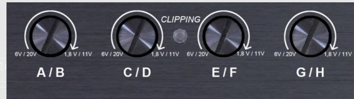
The C-DSP has rotary volume controls for the input sensitivity – the output gain is controlled by the software of the "DSP PC-Tool".
