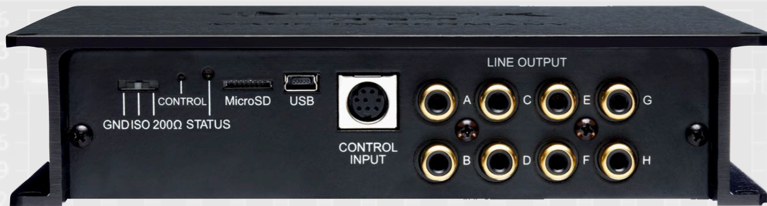
The HELIX DSP offers eight output channels in total – therefore you can find four output pairs (RCA/Cinch; A–H) on its back panel. The routing matrix (see next page) defines which input channel will be allocated to which output channel. Even mixing of several input channels to one output channel is possible.
