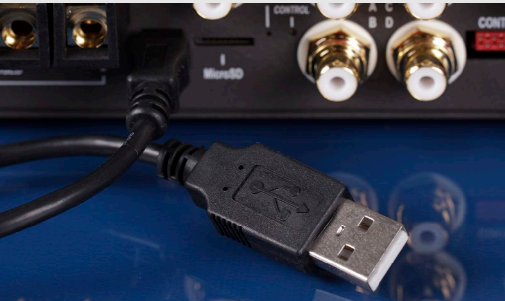
In most cases a USB cable establishes the connection between DSP device and your computer.
