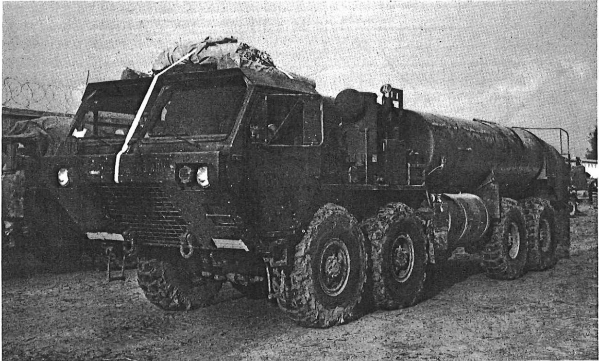
Fig. 10. Heavy Expanded Mobility Tactical Truck (HEMTT) tanker was a primary means of fuel distribution for the 82d Airborne Division.
