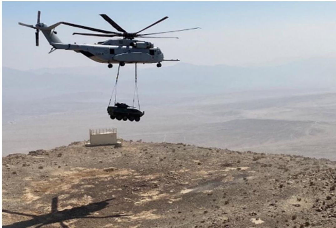
A CH-53K King Stallion conducts an external lift of a LAV-25 (25,200lbs) in the MCAGCC Training Area, Twentynine Palms, CA, at over 8200 feet of density altitude.
