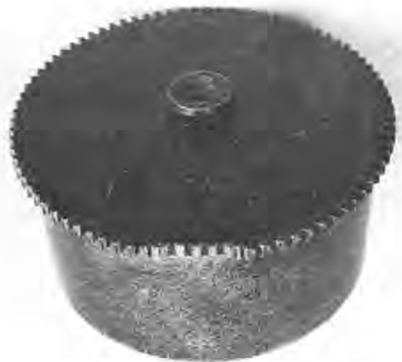
1 A soldered type spring barrel with damaged teeth.
