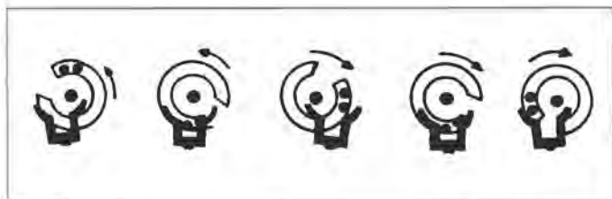
Figure 5. Floating Balance Action
