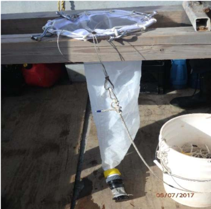
Photograph 23: Zooplankton net set-up prior to deployment on 7 August 2017.
