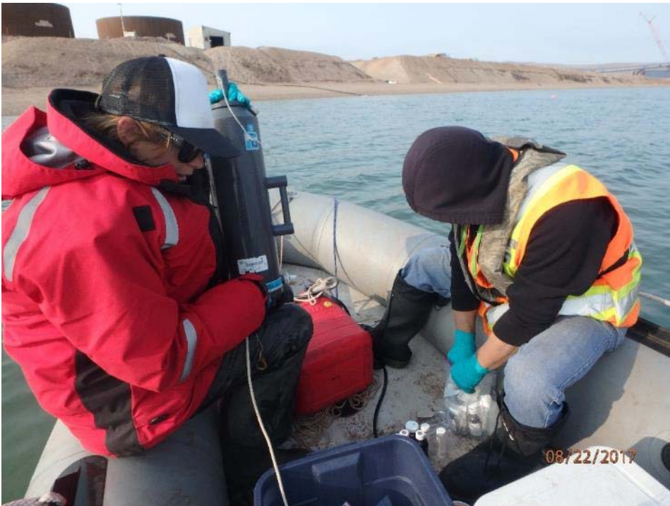
Photograph 4: Collecting water samples using Niskin bottle for water quality analysis on 22 August 2017.
