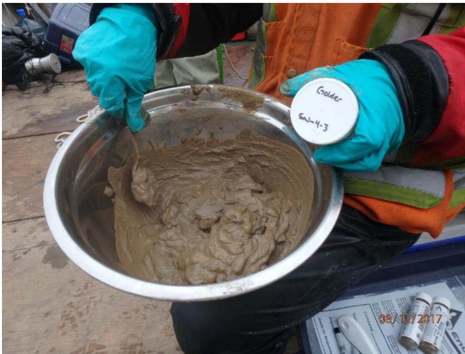
Photograph 8: Stirring sediment to homogenize sample from station SN-4 on 12 August 2017.
