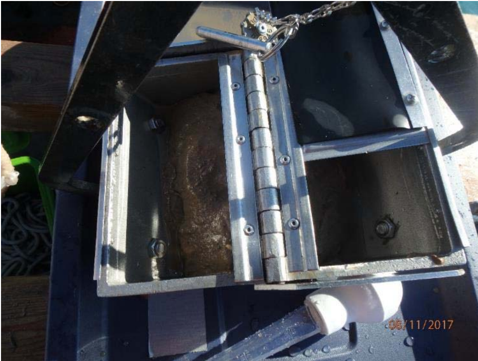
Photograph 5: Open grab sampler, petite ponar, after sediment collection on 11 August 2017.
