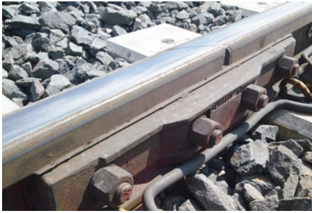
Fig. 2-5: Insulated joint IVB 30° (original) Photo: DB AG/Stefan Ballfanz
