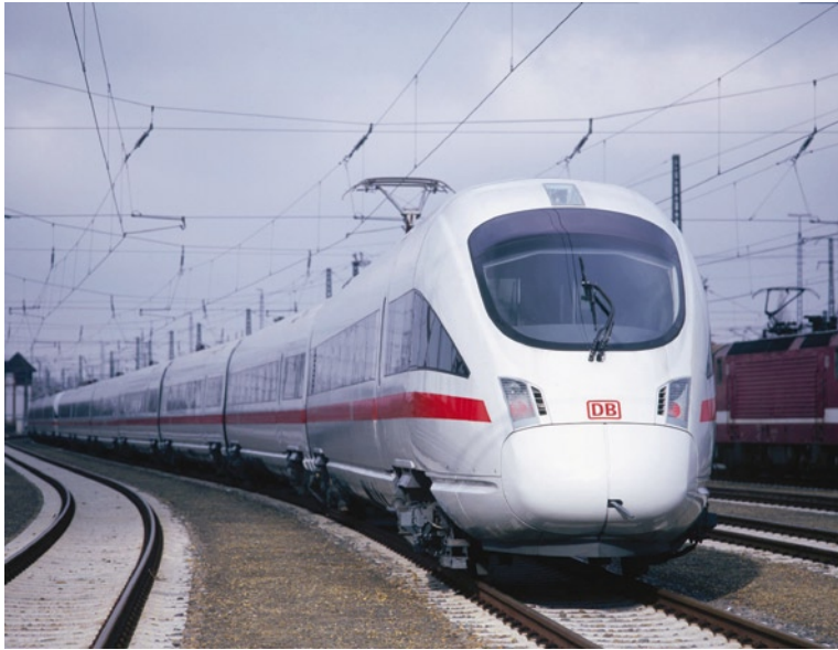
Fig. 1-3: ICE T with body-tilting technology
