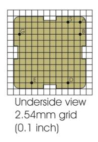
6 holes at 1.6 mm diameter [recommended PCB thickness 1.6 mm]
