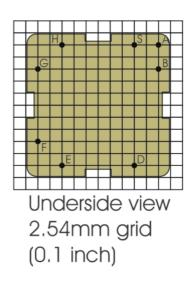
8 holes at 1.6 mm diameter [recommended PCB thickness 1.6 mm]
