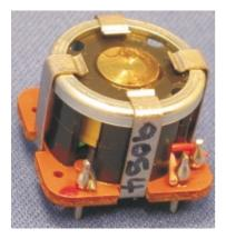
A high performance, professional audio, multi-tapped inductor, intended for line level inductor based equalisation applications.
