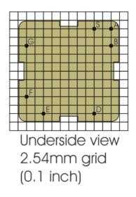
7 holes at 1.6 mm diameter [recommended PCB thickness 1.6 mm]
