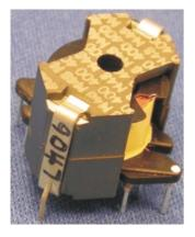
A high performance, professional audio, multi-tapped inductor, intended for line level inductor based equalisation applications.
