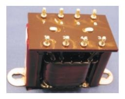
A high performance, ungapped, professional audio signal transformer primarily intended for high level balanced line output applications.
