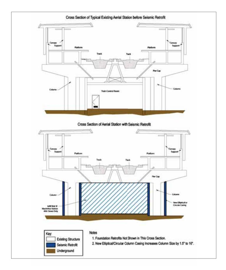
Figure 2-19. Cross-Section of a Typical Aerial Station Before and After Seismic Retrofits
