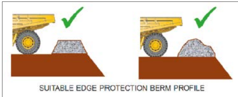
Figure 39 - Example edge protection for tipping operations
