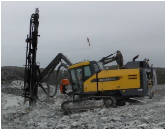
Figure 13 - Example of tracked drilling rig suitable for uneven ground conditions.
