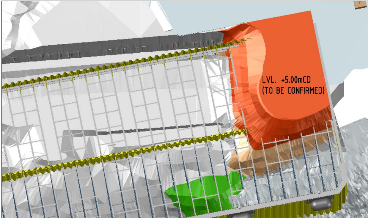
Figure 2 – 3D image showing areas to be blasted underwater and adjacent to the water shown in beige and orange.
