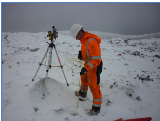
Figure 28 – Surveyor using electronic probe to survey holes
