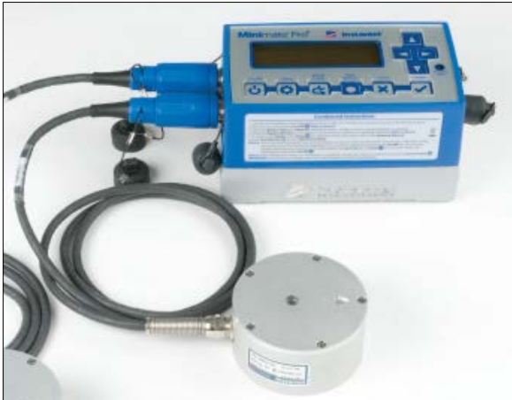
Figure 26 – Example blasting Seismograph for monitoring PPV, air-overpressure, or peak pulse pressure
