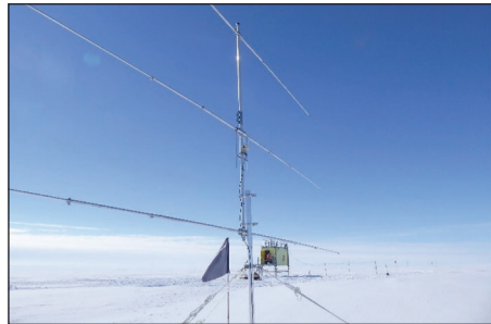
▲ The riometer at Halley Research Station
