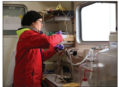
▲ Seawater filtration setup to collect microbial communities. On top of the thin filter membrane, microbes are retained. We fold the filter on the filtration platform, and transfer it to a plastic vial to store it in a -80\text{ }^\circ\text{C} freezer until we extract DNA
