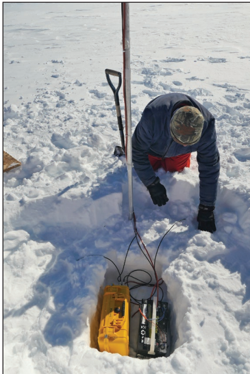
▲ An ApRES (phase sensitive) radar system after being raised during a site-servicing visit on Ronne Ice Shelf
