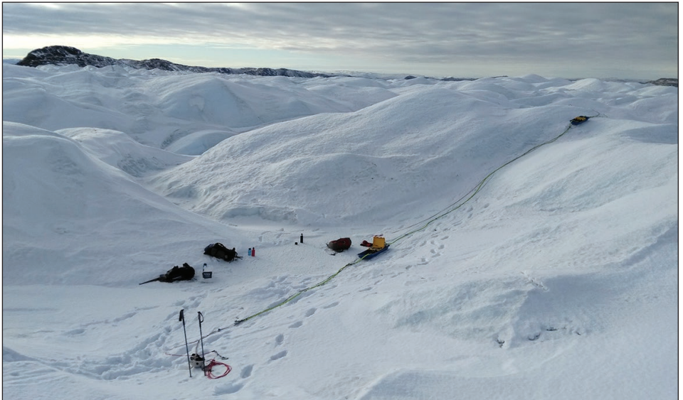
▲ Ice radar system at Leverett Glacier, Greenland with pulks containing radar transmitter and receiver. Green 'hoses' are the radar antennas
