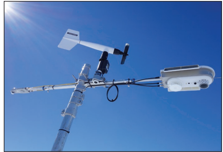
▲ Close up of the sensor yard with on the left the radiation sensors, in the middle the wind speed and direction sensor, and on the right the AWS unit which includes all other sensors except snow temperature
