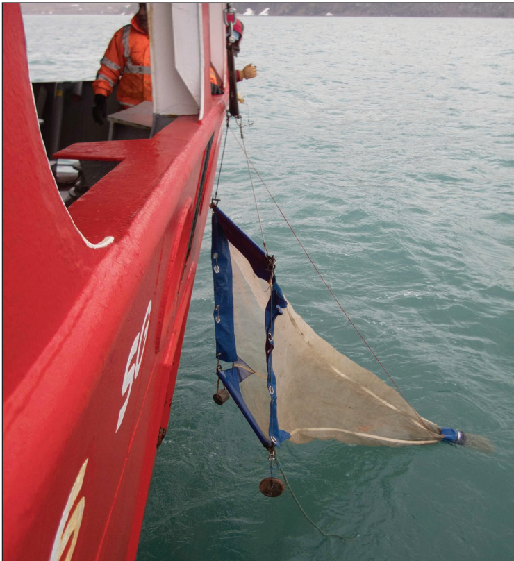
▲ Towing an RMT-I plankton net using the Pharos SG to collect fish larvae and other plankton
