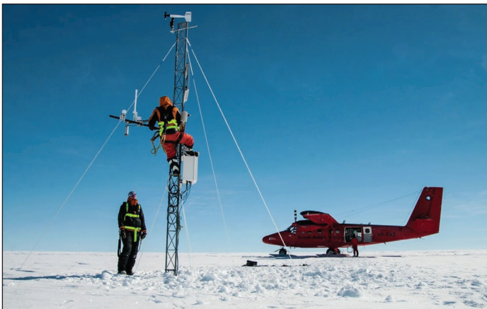
▲ Servicing Butler Island Automatic Weather Station
