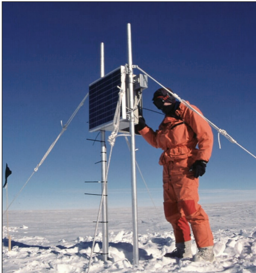
▲ BAS scientist checking the solar power unit for one of the remote low power magnetometers
