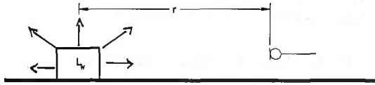
Fig. 2.3 Sound immission at a distance r in free field over reflecting surface
