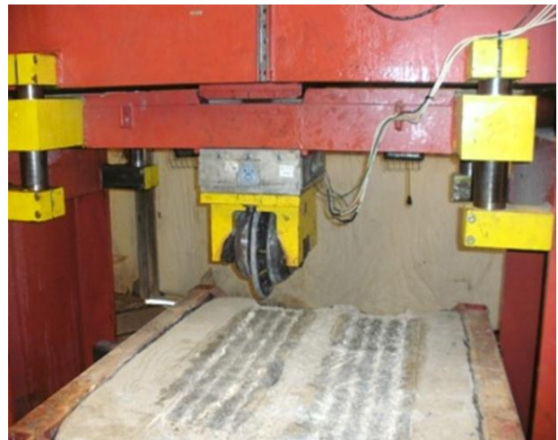
Abbildung 1.5: Linear Cutter Tests
