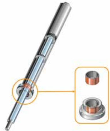
— Figure 3 : Shock absorber sketch with rod guide bush detail
