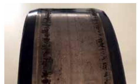
— Figure 2: Local pitting as a result of profiling created by wear
