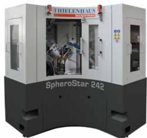
– The new SpheroStar by Thielenhaus Microfinish makes it possible to machine spherical workpieces in short cycle times efficiently and with great precision. photo: Thielenhaus Technologies GmbH
