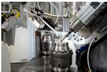
– The SpheroStar has two tool spindle units that can automatically rotate by up to 90 degrees so that the optimal machining position for the relevant process is always selected. photo: Thielenhaus Technologies GmbH
