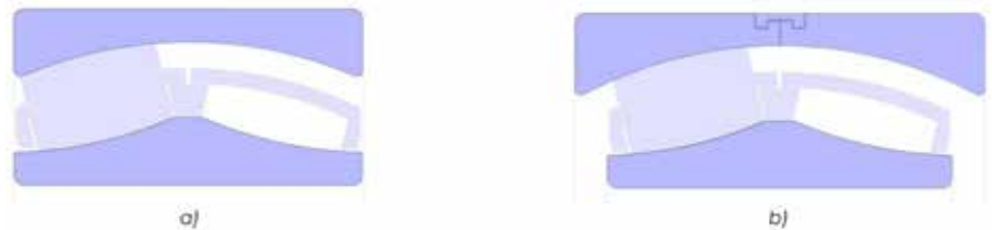
– Fig. 4 – Differences in SRB executions: a) standard design; b) WOR design
