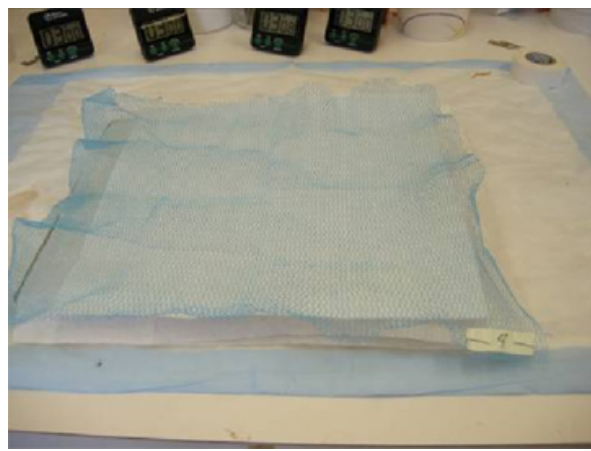
Figure 5.1.4.2.4: Identification of the LLIN. In this example, it is done by stapling masking tape with the barcode number to a corner of the LLIN sample.
