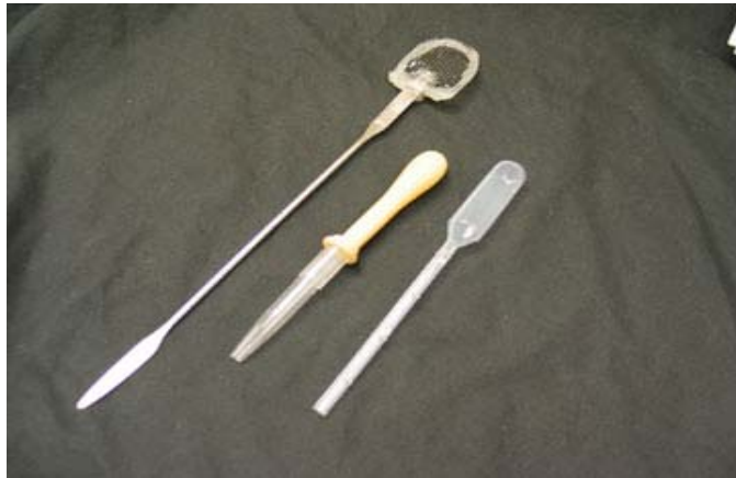
Figure 2.4.7.1. Examples of utensils useful for manual pupae separation or “hand picking”. On the left is a piece of wire mesh glued to a metal spatula and is used to scoop pupae. The middle implement is made of a 1,000 \mu l disposable pipette tip, the tip of which has been trimmed off and fitted with a 2 ml pipette bulb. The pupa picker on the right is a disposable pipette especially good for avoiding contamination as it is transparent. Rinsing these in hot water often is necessary to prevent contamination.
