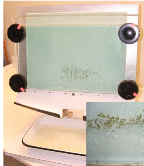
Figure 2.4.7.7. Custom-built pupa separator relying on the size difference between pupa and larva for separation (produced by the John Hock Company).
