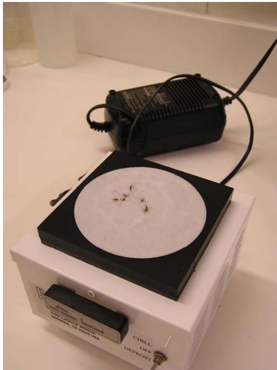
Figure 3.4.2. A small Peltier cold table on which damp filter paper is placed to conduct cold and prevent mosquitoes from sticking to the condensation.
