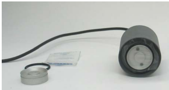
Figure 2.4.10.4. The electric heating unit with a membrane feeder attached to the bottom.
