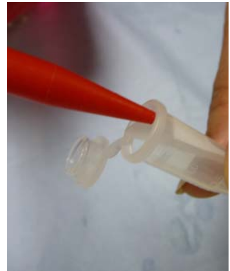
Figure 3.8.3 Moistening the filter paper
