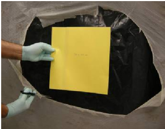
Figure 5.1.4.2.3: Comparison of the size of the template to the size of the sample removed from the LLIN.
