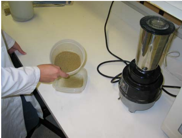
Figure 2.4.6.1. Preparing food. Use a general laboratory grinder (pictured here), a grinding mill or a household coffee grinder. To ensure food is small enough for the earliest stages, use a sieve with holes no larger than 250 microns in size.
