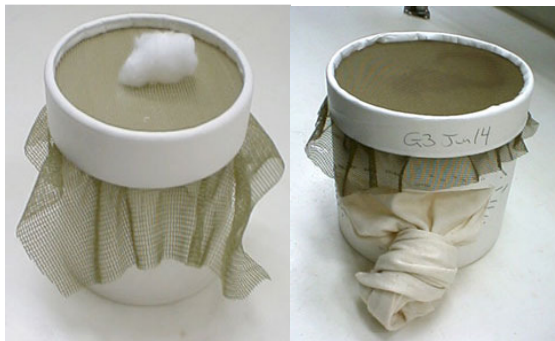
Figure 2.4.8.1. Paper cartons of two sizes, pint (left) gallon (right), showing top entry (left) and side entry (right) solutions.
