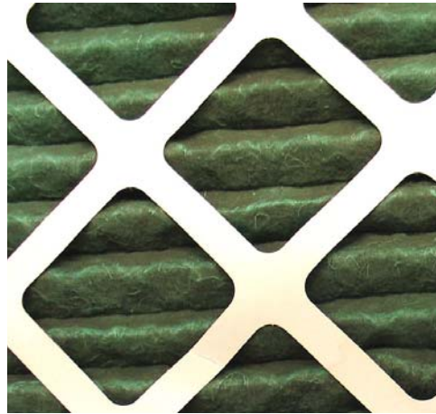
Figure 1.2.3. Dirty air filters are useless or even harmful. Filters should be checked and changed regularly.
