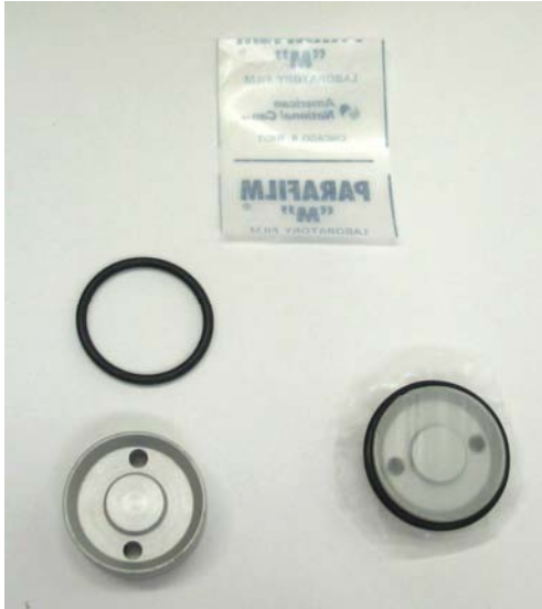
Figure 2.4.10.5. The components that make up the membrane feeder. Clockwise from top, a membrane (in this case Parafilm™; the manufacturer's membranes are recommended), a completely assembled membrane unit ready to be attached to the heating unit, the metal membrane unit without a membrane, and the "O" ring used to attach the membrane.
