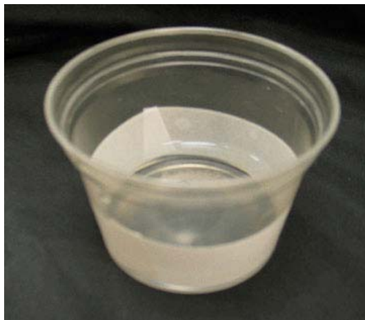
Figure 2.4.1.1. Egg collection cup containing standing water to a depth that is approximately half way up the filter paper liner.
