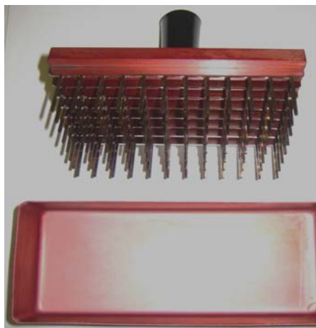
Figure 3.12.1. Example of a 96-bacterial replicator tool used for maceration of mosquito samples and reservoir.
