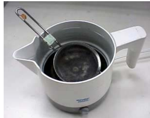
Figure 1.2.1. Any household water-heating pot designed for kitchens can work well in the insectary for sanitizing equipment. Immersing equipment between uses addresses two problems simultaneously: It will clean instruments to protect the transfer of infection and will also kill any larvae/pupae that were accidentally left behind on the tool.
