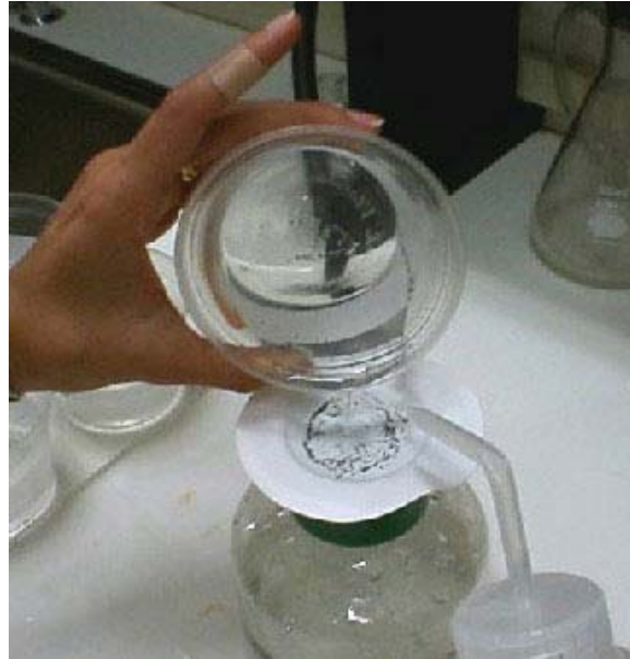
Figure 2.4.2.2 Pour eggs gently into the center of the filtration device. Use bleach solution to remove final eggs from the sides of the container.
