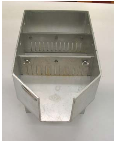
Figure 2.4.7.8. The McCray gate separator. The closest gate to the viewer has a narrower gap than the farthest gate; this is set up to separate dimorphic pupae and larvae.
