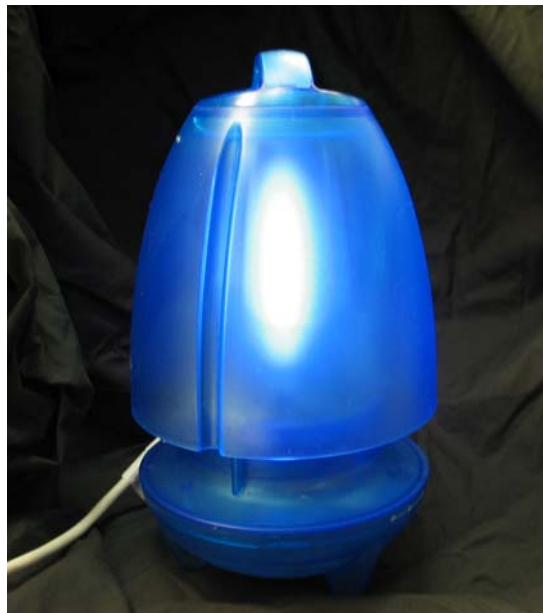
Figure 1.4.5. Light traps, such as the one pictured here, are good for trapping any loose adult mosquitoes. Flying mosquitoes are a serious source of contamination in an insectary and a risk for escaping into the outside environment.
