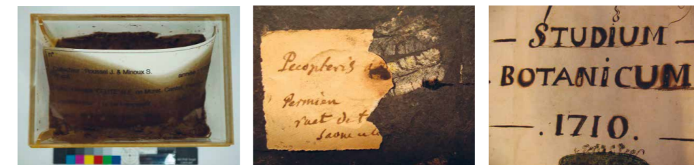
Figure 1. Iron sulfate bearing papers Left: Herbarium front page (Herbier de Fouques, 1710, MNHN); middle : label glued on a fossiliferous shale damaged with sulfate efflorescence (rozenite) (MNHN.F.6890); right : label in contact with a damaged pyritized fossil.
