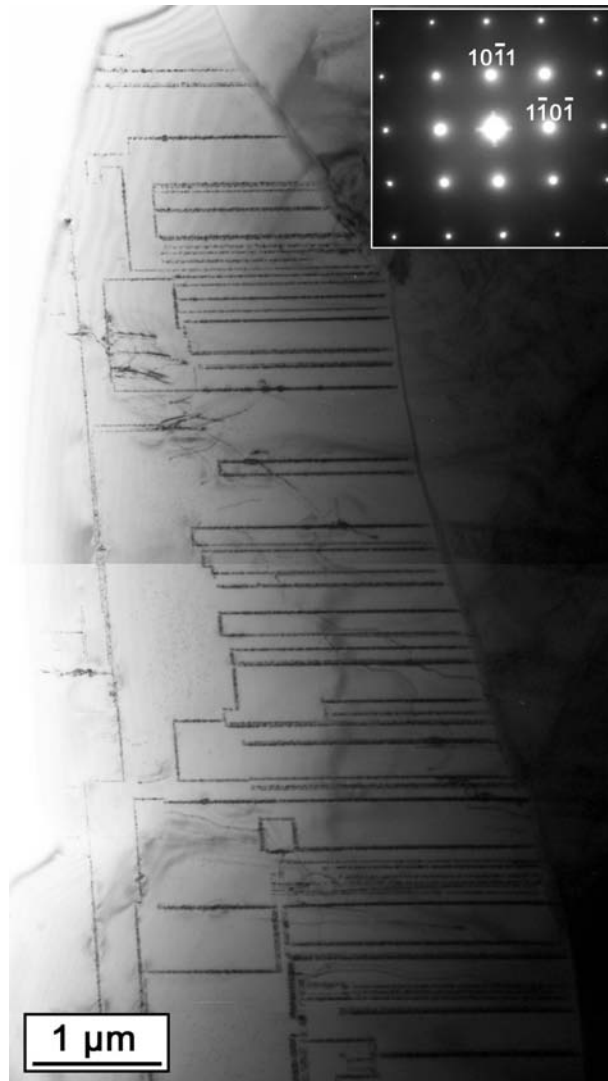
Fig. 3.4-5. Bright-field TEM image of Brazil twins parallel to \{10\bar{1}1\} planes in palisade quartz.
