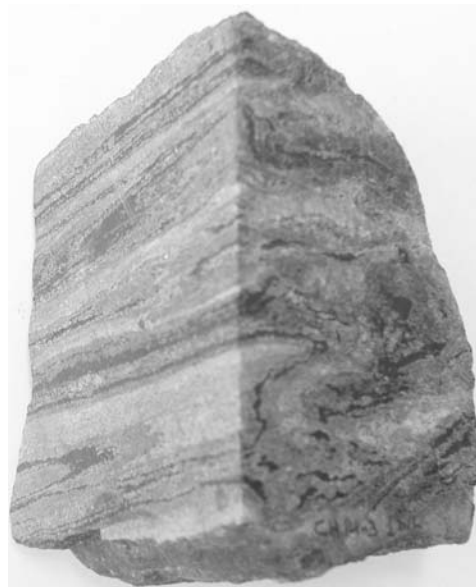
Fig. 3.1-14: Three-dimensional view of the studied sillimanite – garnet – spinel (hercynitic) – quartz gneiss. Sample height is 12 cm.
