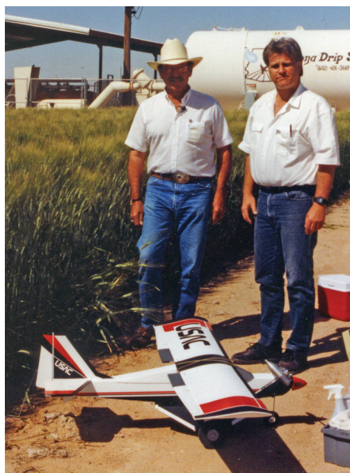
Figure 119. This remote-piloted aircraft releases natural enemies such as green lacewing eggs and Trichogramma , and can treat up to 50 acres. Full-sized aircraft can be used to cover much larger acreages.
