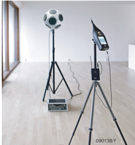
Fig. 10 Optional wireless systems are available to control the sound source for airborne and impact sound insulation measurements
