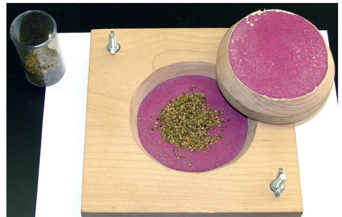
Figure 9. Apparatus used to mechanically scarify prairie clover seed with sand paper. Photo: S. Bushman, ARS.
