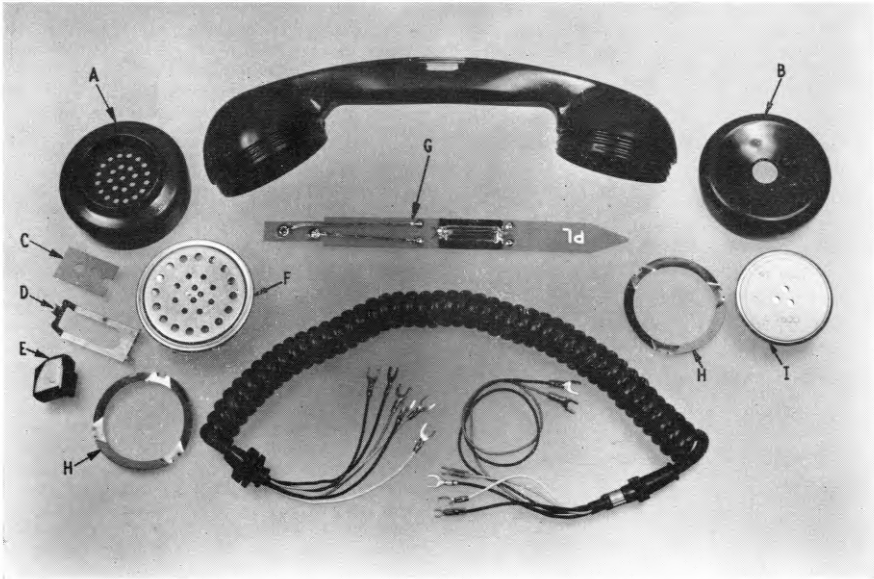
A—Mouthpiece. B—Earpiece. C—S.R.B.P. strip to slot over screw terminals. D—Metal retaining clip. E—Cord-anchor moulding. F—Transmitter. G—Printed-wiring board with neon lamp. H—Spring clips for transmitter and receiver. I—Receiver. Items C and D keep items E and G in position.
