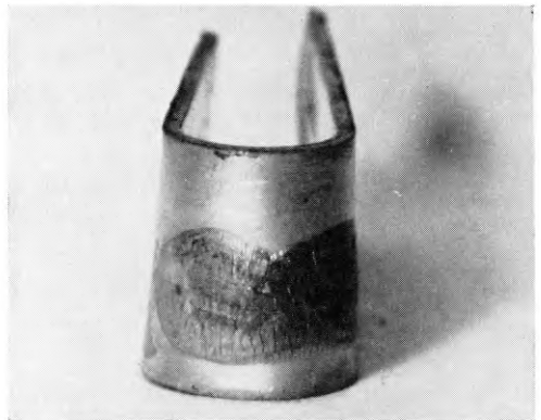
FIG. 3—CRACKS IN SOLDER ON 200-MICROINCH GOLD PLATE
