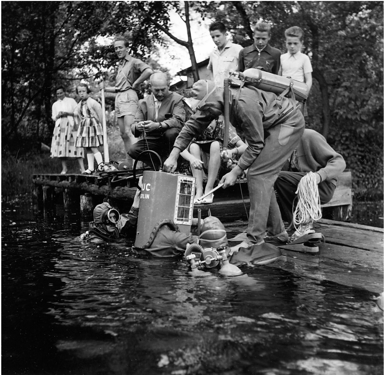
Heinz-Dieter Seiffert, equipped with a "Delphin II" on the jetty. On the right next to the open water diver's helmet is a "Delphin" regulator connected to a twin cylinder diving apparatus and, on the left, a Dräger oxygen rebreather "Model 138" in action. Admired by spectators from the area, a club member is working the lever pump (third from the left on the dock). The safety line for the helmet diver, a reporter from the SFB (Sender Freies Berlin), is held by the trio behind HD Seiffert. Press Photo DUC Berlin, 1957
