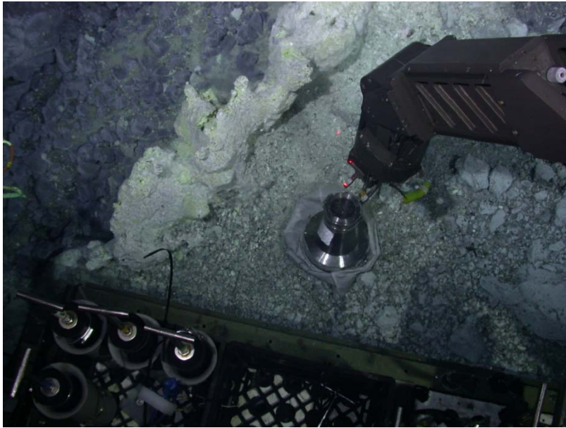
Figure 5.5. Sampling of diffuse fluid using the diffuse flow sampler. The sampler, constructed of Ti, is placed over the area of diffuse flow and a good seal is obtained via careful positioning of the weighted 'skirt' (constructed from a fire blanket). In order to take a sample of the diffuse fluid, the nozzle of the Ti sampler is then inserted into the throat of the diffuse flow sampler. The photograph shown here was taken in the vicinity of the Great Wall at Macintosh Caldera. Note that the 'wall' consists of white and yellow mineral precipitates.
