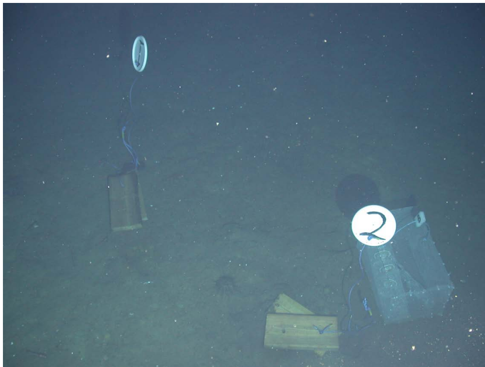
Figure 5.15. Scorpio digital still image of wood-fall substrate units emplaced on seafloor
