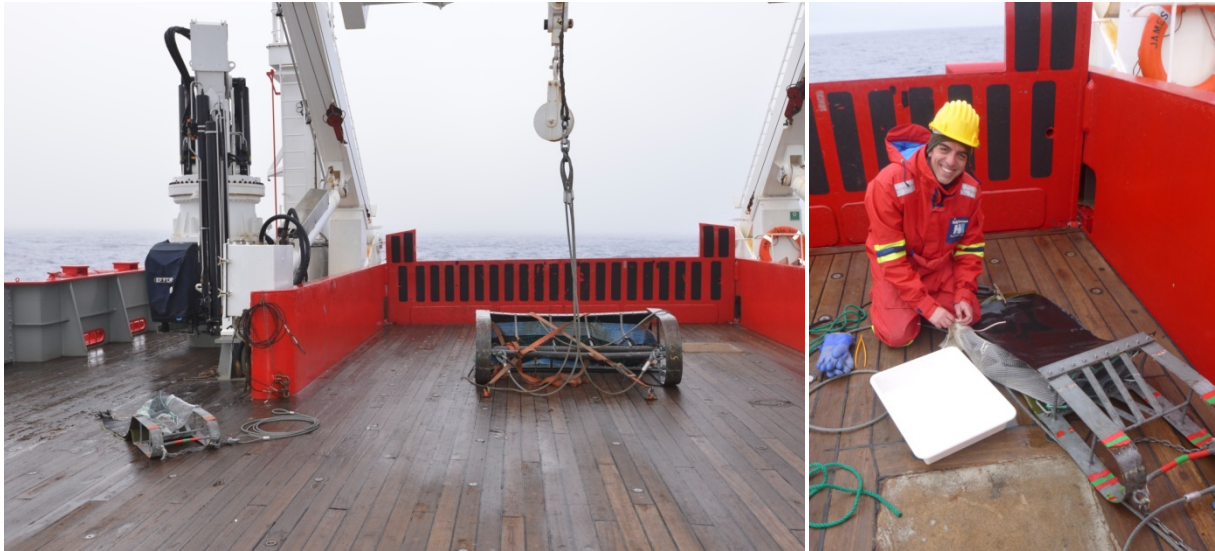
Figure 2.2. Left: Rauschert dredge (left) compared to the Agassiz (centre of deck) on the JCR (© Claudio Ghiglione). Right: Size of the dredge (© Laura Robinson).
