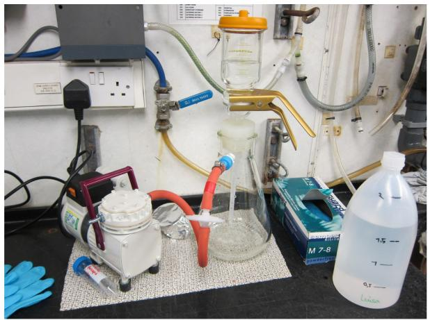
Fig. 25: Setup of filtration unit for analysis of silicon and oxygen isotopes as well as microbial communities in the bottom water (photo: Luisa Federwisch).
