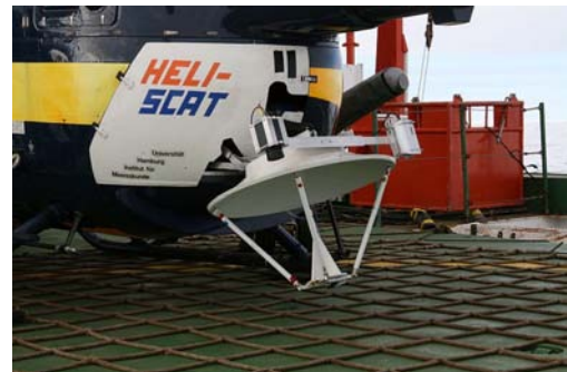
Fig. 3.2.2: Picture of the radar antenna looking out of the helicopter together with the IR camera (to the left above the antenna) and the Video camera (to the right above the antenna)
