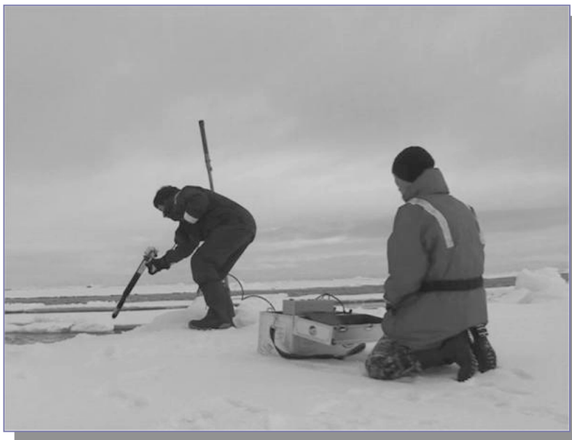
Fig. 4.2.1: XCTD observation on the ice by helicopter operation at XCTD no. 18 on August 17
