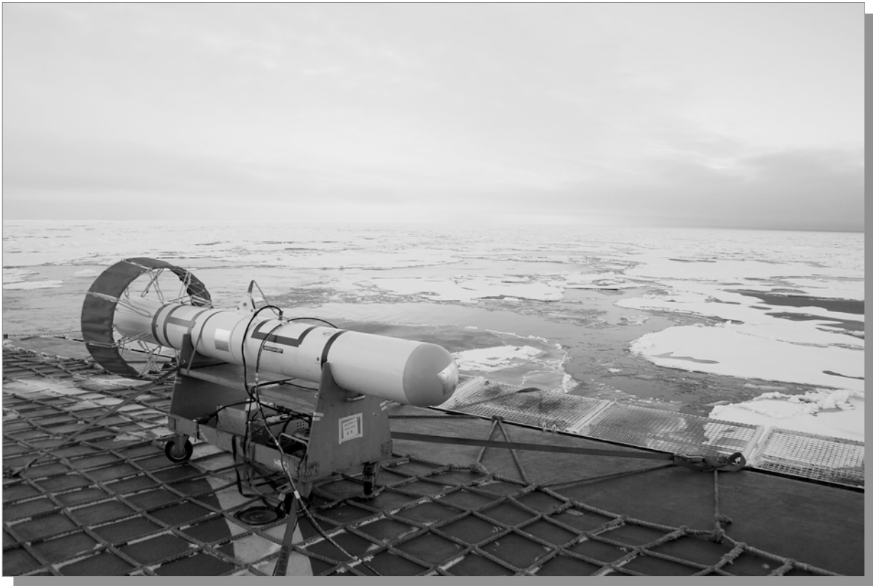
Fig. 3.1.1: EM-Bird on the helicopter deck of Polarstern. A special cart was used for transport, takeoff and landing operations.
