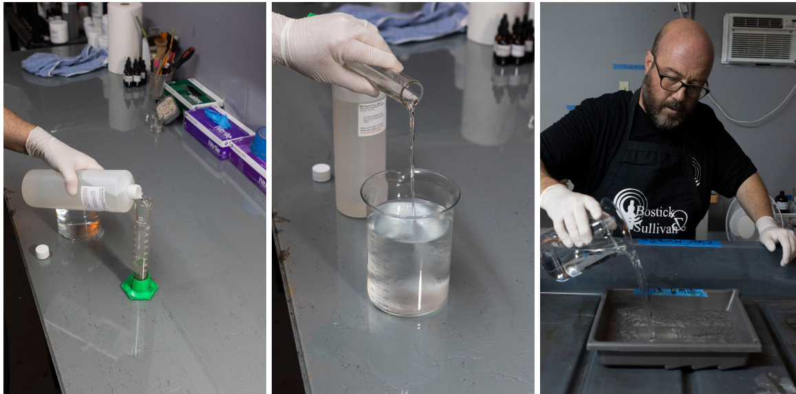
Add 100 ml of Rapid Fixer to 900 ml of cold water to make 1000 ml of working strength fixer.
