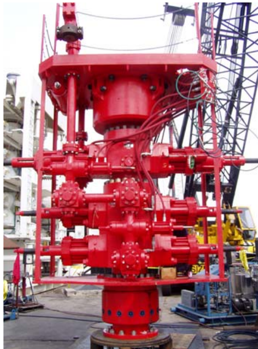
Abb. 6.21: Blowout Preventer (Densley 2012)
