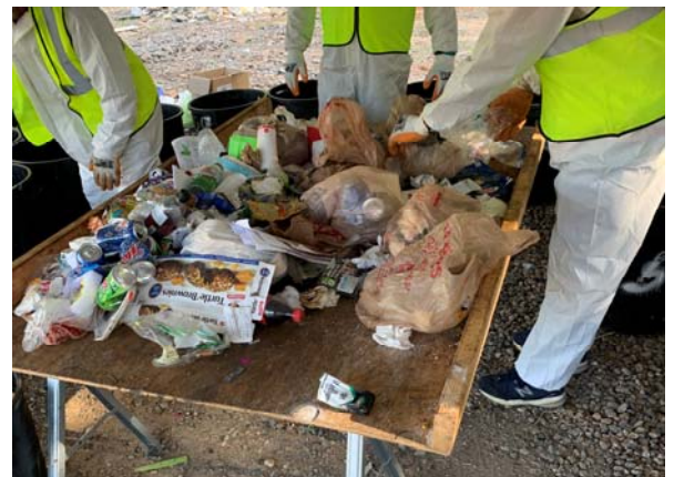
Pictured above: a sample is unbagged and hand-sorted according to material type.
